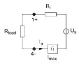
$$\begin{aligned} &R_{load} = \text{Field loop resistance} \\ &U_e = U_s - R_i \times I_e \\ &I_e = U_s / (R_i + R_{load}) \end{aligned}$$
