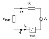
$$\begin{split} &R_{load} = \text{Field loop resistance} \\ &U_e = U_s - R_i \times I_e \\ &I_e = U_s/(R_i + R_{load}) \end{split}$$
