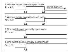
5. A1 -> ∞, A2 -> ∞: Object presence detection mode Object detected: Switch output closed No object detected: Switch output open
