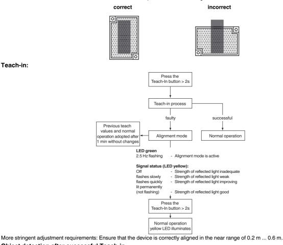
**Object detection after successful Teach-in** The target should be large enough so that the reflector is always completely covered in one dimension!
