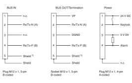
According to the "PROFIBUS Mounting Recommendations", the connection of the screen with Pin 5 is not recommended if necessary, this type connection should be chosen if the contact of the screen cannot be established by screwing it to the plug housing.
