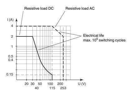
The maximum number of switching cycles is depending on the electrical load and may be higher when reduced currents and voltages are applied.
