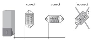
The edge of the sensor must be parallel with the edge of the reflector!
