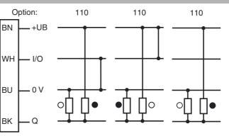
The circuitry for the external input applies to the master and all connected slave modules
