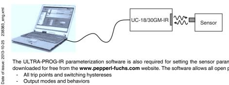
The ULTRA-PROG-IR parameterization software is also required for setting the sensor parameters. The ULTRA-PROG-IR software can be downloaded for free from the www.pepperl-fuchs.com website. The software allows all open parameters to be set, including:
