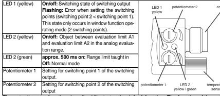
The potentiometer function described illustrates the default function. The function of the potentiometer can be altered using the ULTRA-PROG-IR software. As soon as a configuration has been changed, the potentiometer function selected using ULTRA-PROG-IR is activated.
