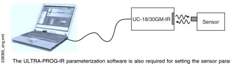
The ULTRA-PROG-IR parameterization software is also required for setting the sensor parameters. The ULTRA-PROG-IR software can be downloaded for free from the www.pepperl-fuchs.com website. The software allows all open parameters to be set, including:
