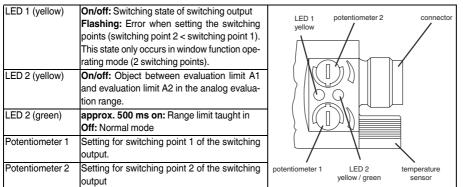
The potentiometer function described illustrates the default function. The function of the potentiometer can be altered using the ULTRA-PROG-IR software. As soon as a configuration has been changed, the potentiometer function selected using ULTRA-PROG-IR is activated.
