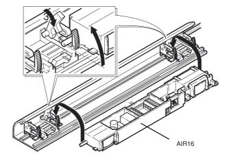
Sensors can be replaced faster and more easily with the locking mechanism on the print holder.
