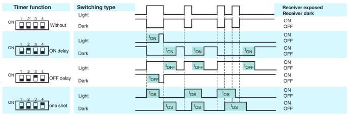
Time  $t_{ON}$ ,  $t_{OFF}$  and  $t_{OS}$  are adjustable from 0.02 to 1 seconds. The Light-/Dark-Switch (Left, outer switch) is shown in the "Dark ON" position.
