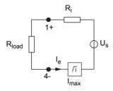
$R_{load}$  = Field loop resistance  $U_e = U_s - R_i \times I_e$  $I_e = U_s/(R_i + R_{load})$
