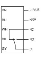
The relay-functions "NC" and "NO" bear on the switching mode "Light-ON". This complies to the default setting of the light/dark switch, located on top of the housing (factory setting).
