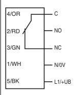
The relay-functions "NC" and "NO" bear on the switching mode "Light-ON".
