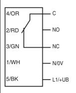
The relay-functions "NC" and "NO" bear on the switching mode "Light-ON". This complies to the default setting of the light/dark switch, located on top of the housing (factory setting).
