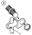
① Fasten the two parts of the ② mounting clamp (a) loosely by means of the screw (b) and the nut (c) supplied.
