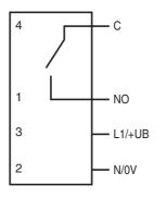
The relay-functions "NC" and "NO" bear on the switching mode "Dark-ON".
