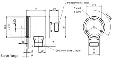
$^{\star}$  with axial exit position L 42, with radial exit position L 53  $^{\star\star}$  Aluminium: d = 59, stainless steel: d = 61
