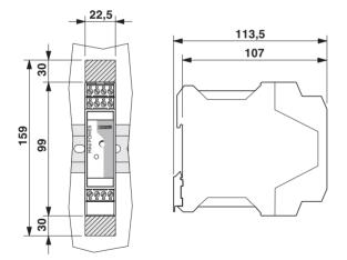
Installation: Installation depth 95 mm (+ DIN rail)
