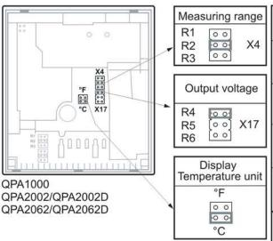
Set either X4 or X17 into test function, but not both at the same time.
