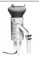
• This detector tester contains a hot air generator. For the performance check, the tester is pushed over the detector. The hot air released heats the detector and so actuates an alarm.
