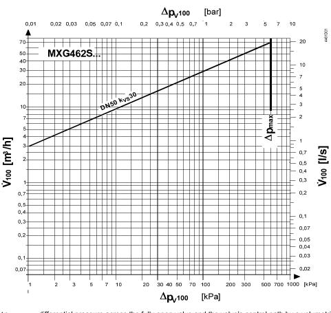
$\Delta p_{v100}$  = differential pressure across the fully open valve and the valve's control path by a volumetric flow V<sub>100</sub>
