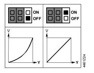
Output signal U (position feedback signal) is dependent on the load resistance Ri.
