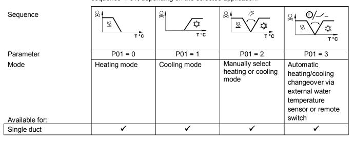
In application "Single duct with el. heater", the controller operates in heating AND cooling mode.
