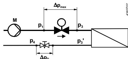
**Удалено:** Cavitation accelerates wear on the valve plug and seat, and also results in undesirable noise. Cavitation can be avoided by not exceeding the differential pressure shown in the flow diagram on page 5 and by adhering to the static pressures shown below.
