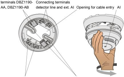
Connecting terminals detector Mounting slots min. 40 mm up to max. 90 mm line and ext. Al
