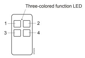
Overview of display and operating element functions on the AFK914/C01:
