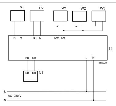
P1, P2 Third-party meter with potential-free pulse contact, e.g. for hot water, chilled water, electricity, etc. W1...W3 Heat meter
