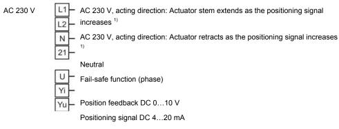
Positioning signal DC 0...10 V
