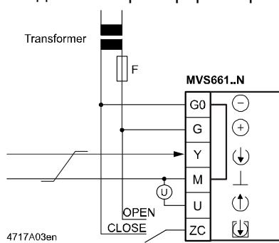
**Terminal assignment for controller with 3-wire connection**
