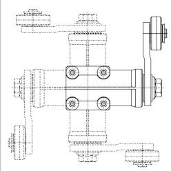
The actuating head can be repositioned by  $4 \times 90^{\circ}$ . Unscrew the four screws of the actuating head, reposition the actuating head in the desired position and retighten the four screws.
