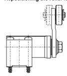
The (offset) roller arm may be reversed, so that the roller faces the inside of the arm.
