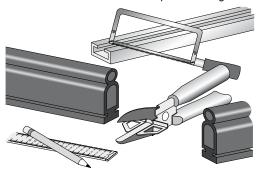
2. If necessary, pull the safety edge slightly out of the aluminium profile or drill mounting holes; max. hole distance 70 mm; fix the aluminium profile by means of oval-head or countersunk head screws Ø 3 ... 6 mm.
