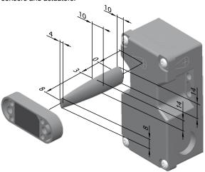
Assured switching distance:  $s_{ao} = 8 \text{ mm}$ Assured switch-off distance:  $s_{ar} = 18 \text{ mm}$
