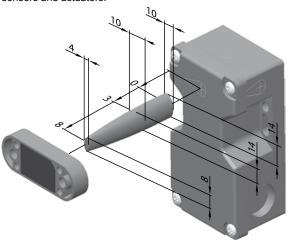
Assured switching distance:  $s_{ao}$  = 8 mm  $s_{ar}$  = 18 mm Assured switch-off distance:
