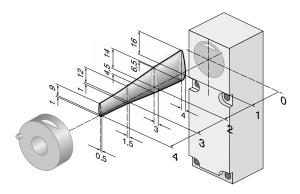
Assured switching distance:  $s_{ao} = 4 \text{ mm}$ Assured switch-off distance:  $s_{ar} = 14 \text{ mm}$
