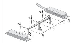
assured switching distance:  $s_{ao} = 8 \text{ mm}$ assured switch-off distance:  $s_{ar} = 18 \text{ mm}$
