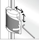
Step 6 Press down the handle, so that it latches. Accurately align the handle unit with the sensor. Tighten the handle unit using the supplied hexagonal key.
