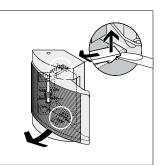
Step 3 Remove the spring from the handle. Loosely tighten the handle unit Use screwdriver to remove the handle
