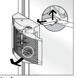
Step 4 Remove the handle using a screwdriver, unscrew the device (if necessary) Procedure for fixing: refer to first assembly
