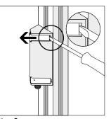
Step 2 Remove the plates of the sensor using a screwdriver, unscrew the device (if necessary)
