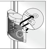
Step 3 Remove the spring from the handle.
