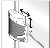
Press down the handle, so that it latches. Accurately align the handle unit with the sensor. Tighten the handle unit using the supplied hexagonal key.
