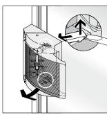
Remove the handle using a screwdriver, unscrew the device (if necessary) Procedure for fixing: refer to first assembly
