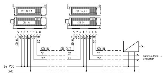
Y1 and Y2 = Safety outputs Safety monitoring module SD-IN -> SD-i-DP = PROFIBUS
