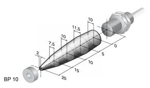
Assured switching distance:  $s_{ao} = 10 \text{ mm (BP 6 / BP 8)}$
