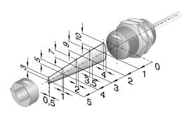
Assured switching distance: Assured switch-off distance
