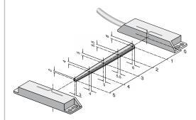
Assured switching distance:  $s_{ao} = 5 \text{ mm}$ Assured switch-off distance:  $s_{ar} = 15 \text{ mm}$
