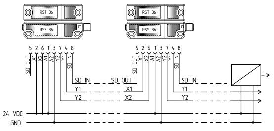
Y1 and Y2 = Safety outputs  $\rightarrow$  Safety monitoring module SD-IN  $\rightarrow$  Gateway  $\rightarrow$  Field bus
