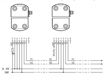
Y1 and Y2 = Safety outputs → dual-channel safety monitoring module
