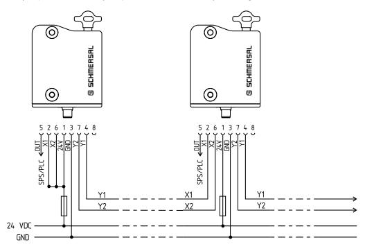
Y1 and Y2 = Safety outputs  $\rightarrow$  Safety monitoring module
