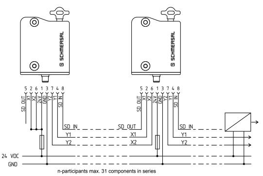
Y1 and Y2 = Safety outputs  $\rightarrow$  Safety monitoring module SD-IN  $\rightarrow$  Gateway  $\rightarrow$  Field bus
