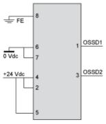
With External Device Monitoring (EDM) feedback loop
