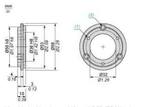
3 holes M4 x 0.7 at 120° on 42 PCD. TC M3 x 8 screw fixings 3 counterbored holes for TC M4 x 8 screws at 120° on 48 PCD (1) (2)
